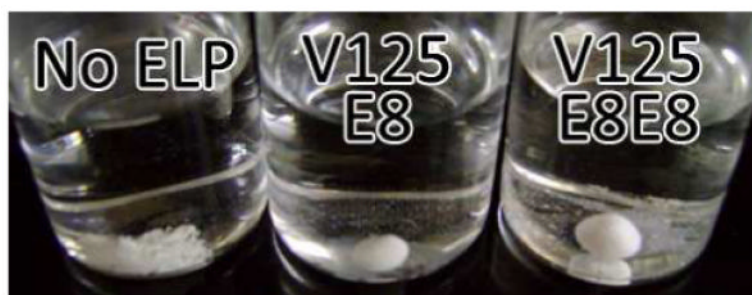
Figure 6. Washout studies of ELP and CPC composites
