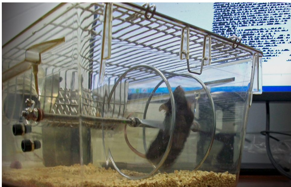
In this study, the mice’s running activity was monitored via a direct data link to a computer running Clocklab™ Analysis software. Mice that exercised before PCB exposure showed fewer changes to the gut microbiome than sedentary mice.
