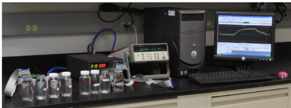
Fig. 6. Photograph of the testing apparatus used to determine sensor electrical output characteristics. The sensors were placed in solutions of varying ionic strength and the voltage output was simultaneously measured.
