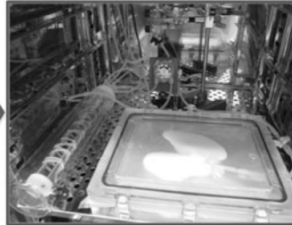
Fig. 2. Representative images of porcine livers during decellularization process and the closed perfusion system
