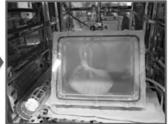
Fig. 2. Representative images of porcine livers during decellularization process and the closed perfusion system
