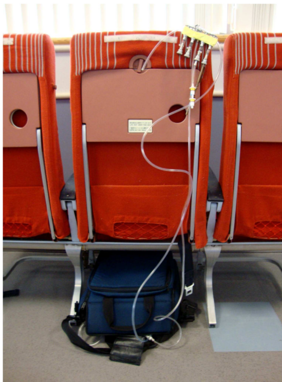
Figure 1. Sampling system for the ozone monitor, sorbent tubes and pumps on/under an aircraft seat.
