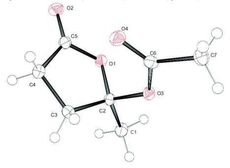
**Figure 1** *ORTEP* (Farrugia, 2012) view of the title molecule showing the atomic numbering and 50% probability displacement ellipsoids.
