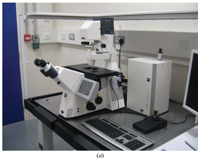
Figure 1 PALM MicroTweezers microscope (Zeiss). (a) Overall view. (b) Sample environment with SmarAct micromanipulators for sample holders.
