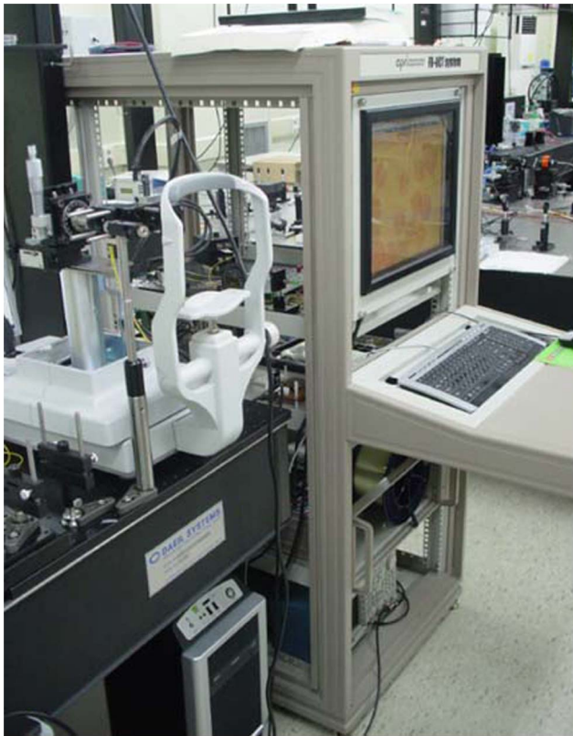
Figure 2. A photograph of the Fourier-Domain OCT (optical coherence tomography) used in this study. doi:10.1371/journal.pone.0067143.g002
