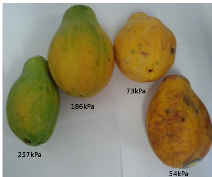
Figure 14. Turgor pressure in Kilo-Pascal (kPa) measured with the glove for papaya. The fruit on the left is more unripe and the one on the right is more ripe.
