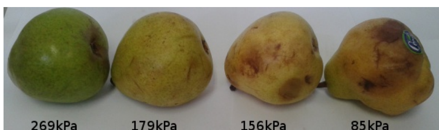
Figure 11. Turgor pressure in Kilo-Pascal (kPa) measured with the glove for peach. The fruit on the left is more unripe and the one on the right is more ripe.
