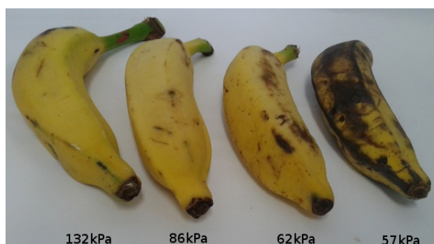
Figure 15. Turgor pressure in Kilo-Pascal (kPa) measured with the glove for banana. The fruit on the left is more unripe and the one on the right is more ripe.
