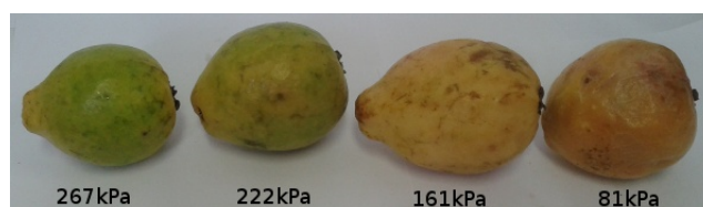
Figure 16. Turgor pressure in Kilo-Pascal (kPa) measured with the glove for guava. The fruit on the left is more unripe and the one on the right is more ripe.
