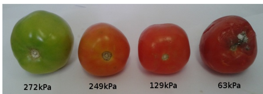
Figure 12. Turgor pressure in Kilo-Pascal (kPa) measured with the glove for tomato. The fruit on the left is more unripe and the one on the right is more ripe.
