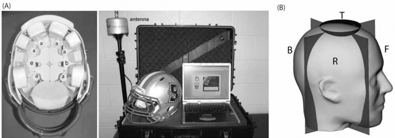
Figure 1. Football players wore helmets instrumented with the HIT system that was specifically designed to record head accelerations as a result of an impact to the helmet without interfering with play. The HIT System (A) comprises an in-helmet unit containing six accelerometers (a), battery (b), transmitting and logging electronics (e), a sideline receiver, and a laptop computer. An illustration (B) of the regions that defined the front (F), right side (R), back (B) and top (T) helmet impact locations.
