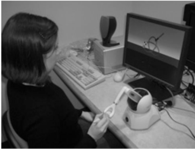
Figure 1. A) Example of display and target path. B) The Phantom together with the display.
