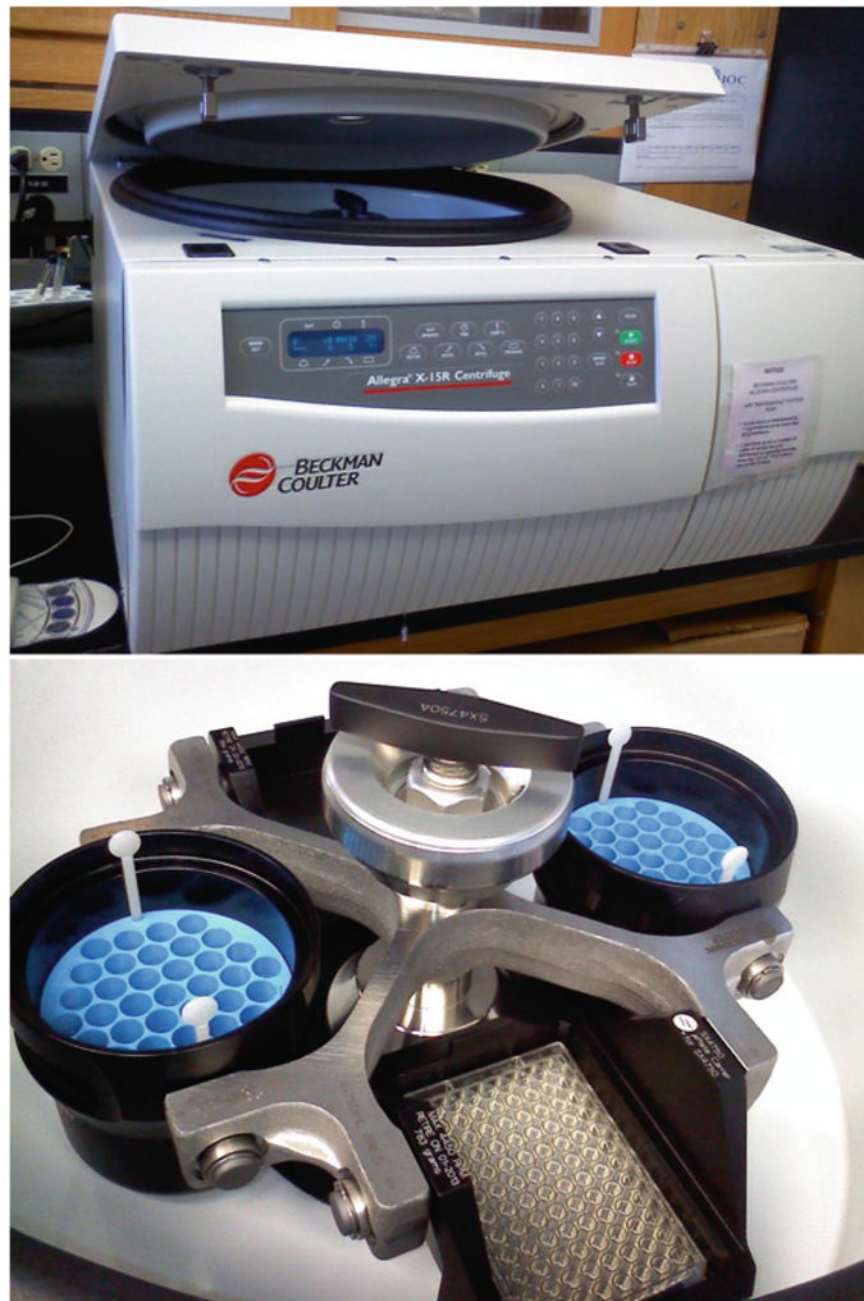
Fig. 2. Example of a low-speed centrifuge with adapter for spinning AggreWell plates.
