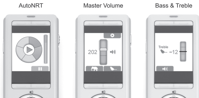
Figure 2. Remote Assistant Fitting on the Nucleus CR110 Remote Assistant. Left: AutoNRT in progress on the second of five electrodes. Middle: Master Volume adjustment. Right: Treble adjustment.
