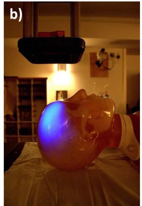
Fig. 3. (color online) The gated detection of Cerenkov emission with room lights on is shown with spectra acquired from a scattering phantom, left. The Cerenkov emission is obtained by calculating the difference between the gated signal and ambient lighting signal. A photograph of the room with a corresponding image of Cerenkov emission from the scattering phantom are overlaid to illustrate the amount of ambient lighting present for all experiments.
