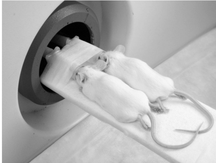
Figure 4. Illustration of simultaneous side-by-side imaging of two mice with the VISTA scanner. For size reference, the bore diameter of the VISTA machine is 8 cm.
