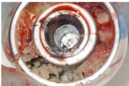
Figure 5 Macroscopic wear of the taper.
