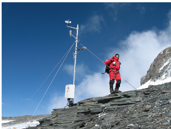
Figure 1 Automatic weather station as installed at the South Col of Mount Everest in May 2008.
