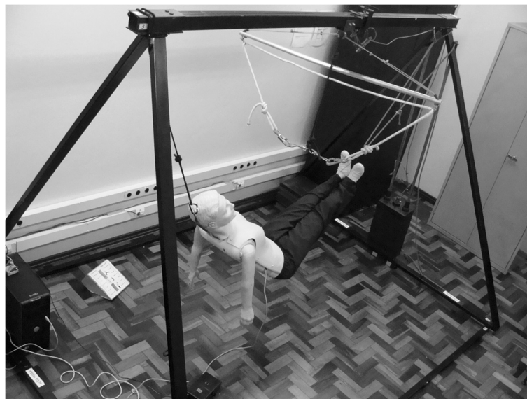
Figure 1 Body suspension device with mannequin fully suspended simulated microgravity.
