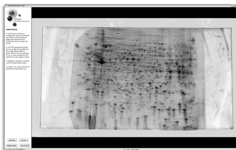
Fig. 1. Gel image cropping with the RAIN submission tool. The shaded area shows an optimum polygonal crop that removes the gel edges and some artifacts while retaining the protein spots
