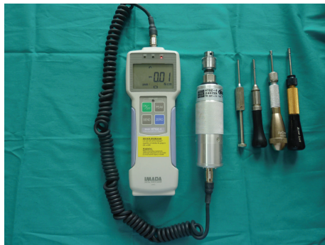
FIGURE 4: Portable digital torque gauge and screwdrivers.
