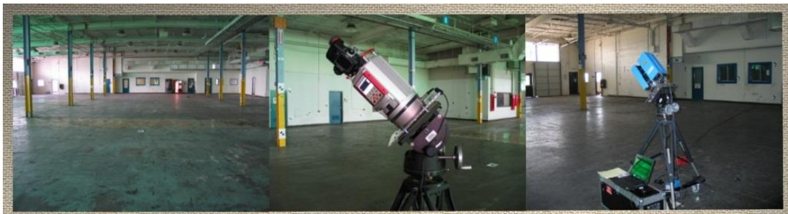
Figure 16. TLS user self-calibration field setup with a Riegl VZ-400 and Z+F Imager 5003 at the University of Houston.
