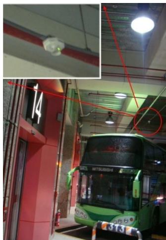
Figure 9. The actual ultrasound transmitter is located approximately 1m from the buses.
