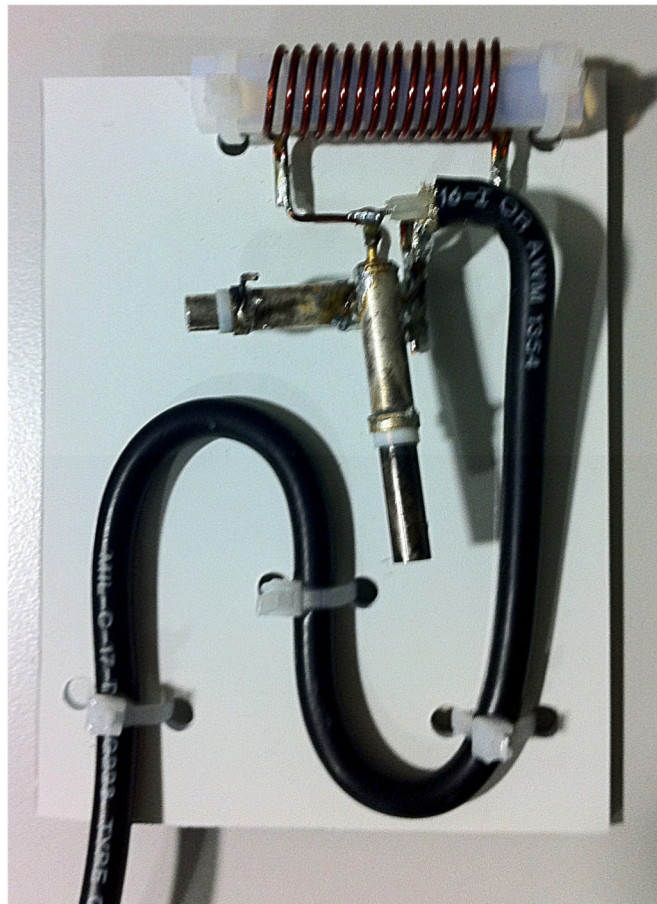
Figure 1. Example standardized RF coil used at field strengths from 1.5 T to 7 T. Coils are transmit/receive parallel dual-conductor solenoids.
