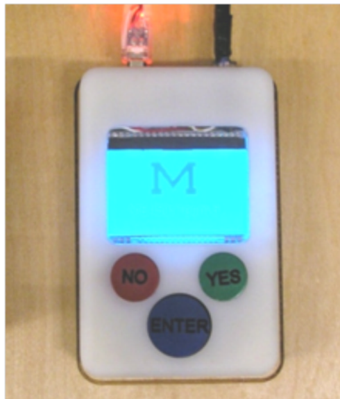
Figure 3. A. Exploded view of prototype PCA patient handset. B. PCA prototype handset with liquid crystal display (LCD) screen.
