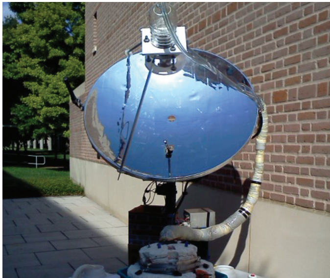
Standalone solar autoclave with parabolic dish collector.
