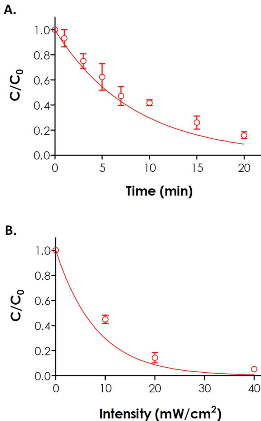
**Fig. 4.** (A) Effect of UV irradiation time (365 nm,  $10 \text{ mW}/\text{cm}^2$ ) on peptide photolysis. Symbols represent experimental results while the exponential decay curve is a prediction using Eqs. (1) & (2). (B) Effect of UV light intensity (365 nm, 10 minutes) on peptide photolysis. Symbols represent experimental results while the exponential decay curve is a prediction using Eq. (3).
