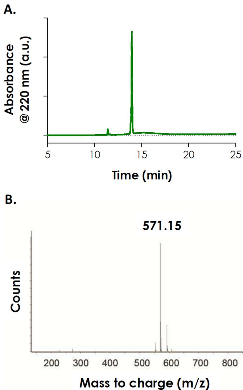
**Fig. 1.** (A) HPLC trace of purified photodegradable peptide Ac-CGOGC-NH<sub>2</sub>. (B) Mass-spec result of purified photodegradable peptide (peptide expected exact mass: 571.15 Da).
