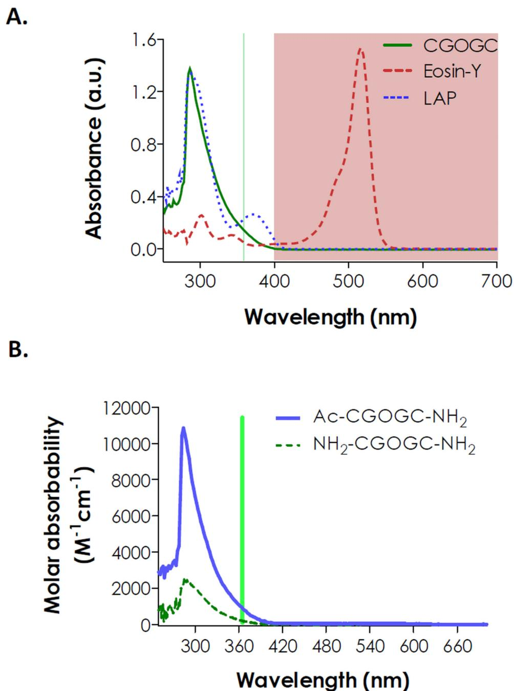
**Fig. 2.** (A) UV/Vis absorbance spectra of photodegradable peptide, visible light initiator eosin-Y, and UV light initiator LAP (Shaded area indicates visible light absorbance range). (B) Effect of peptide N-terminal acetylation on molar absorptivity measured in 10% (v/v) DMSO aqueous solution. Vertical line indicates a wavelength (365 nm) commonly used for UV-mediated reactions.
