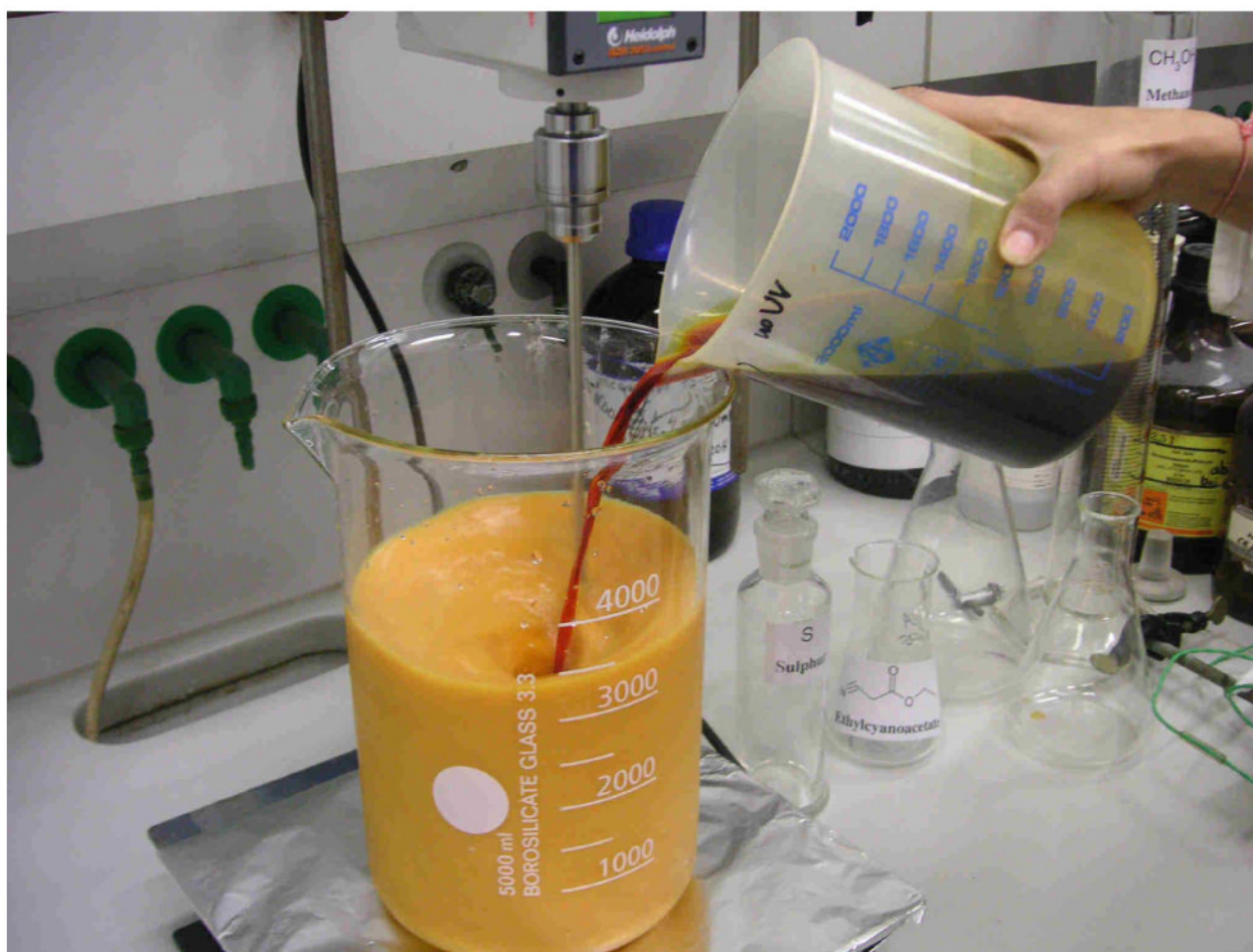
Figure 1. Simple to perform large scale open vessel Gewald-3CR (courtesy of Prof. Ulrich Jordis, Vienna).
