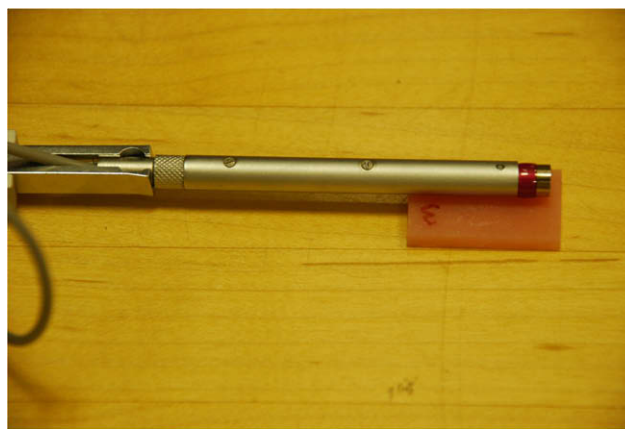
Figure 2 Perthometer recording the surface roughness of acrylic resin specimen.
