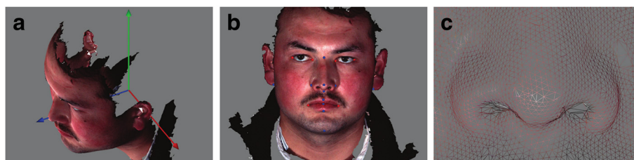
Figure 1 The surface used in our research. (a) The coordinate system used in our research (red, green and blue axes stand for x, y and z axes respectively). (b) An example scan with 17 landmarks marked by the colored spots. The red spots are the 6 most salient landmarks, namely the inner and outer corners of the eyes and both corners of the mouth, the blue spots indicate the other 11 landmarks used in this study. (c) Raw mesh details around the nose tip.
