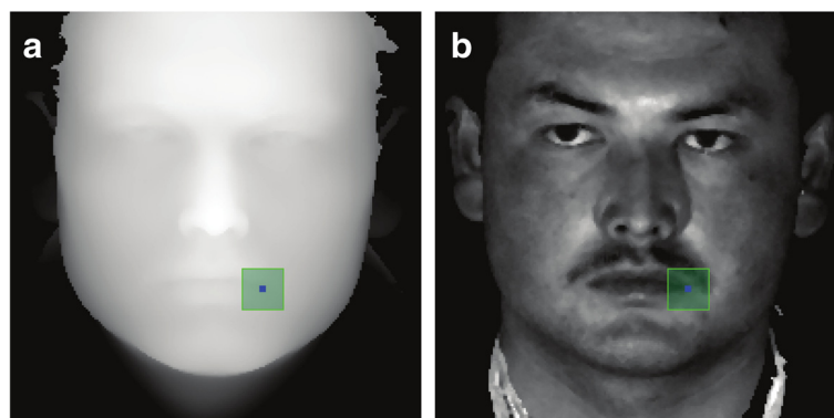
Figure 4 The signature patch for the left lip corner illustrated in the 2D space. (a) The z coordinate values mapped into the 2D space. (b) The gray scale values mapped into the 2D space.
