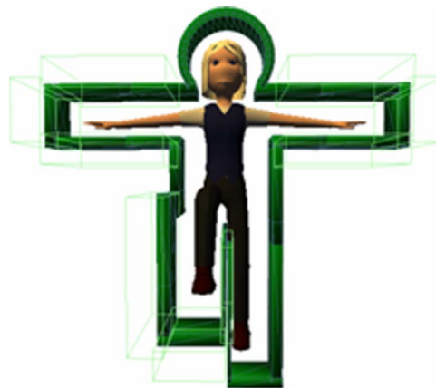
Figure 12. Detection of collisions between the avatar and the posture frame. doi:10.1371/journal.pone.0069471.g012
