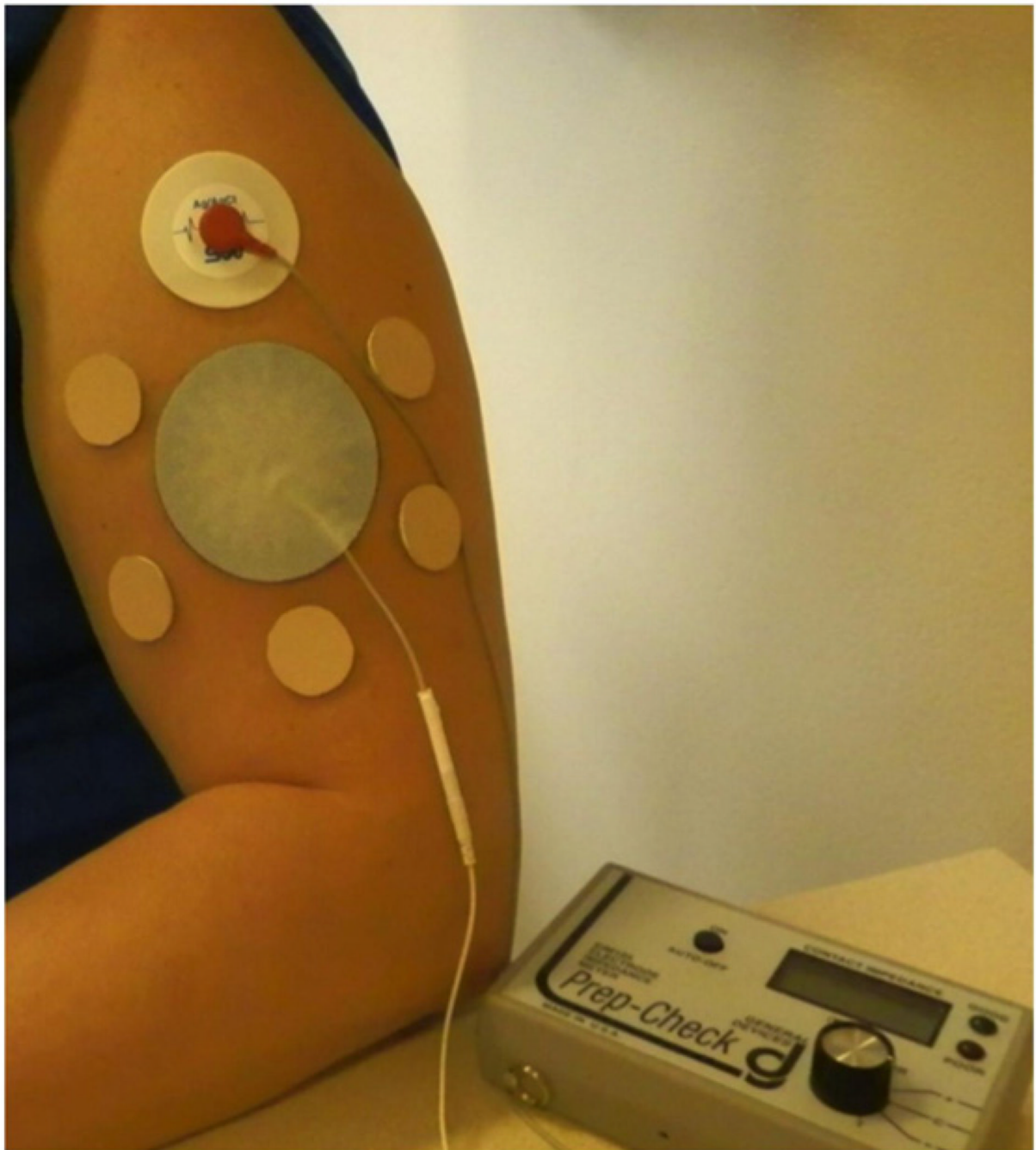
Fig. 2. Treatment patches and electrodes on a subject's upper arm. The reference electrode was placed in the middle of all the treatment sites, which were protected during the study by blank occlusive patches. The top treatment site displays one of the Ag/ AgCl measurement electrodes, which is moved from site to site to make impedance measurements. Both the reference and measurement electrodes are connected by lead wires to the impedance meter.
