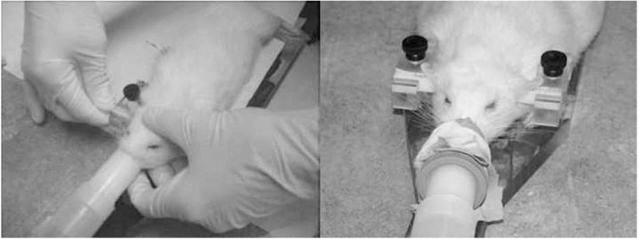
Fig. 10. Keeping a rat under anesthesia while inserting ear bars. Detachable bite bar assembly was removed to improve maneuverability while inserting earbars, and to enable direct connection of the anesthesia line to the rat via a nose cone.
