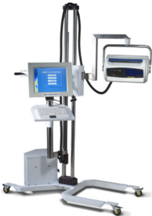
Figure 6. Laser Doppler imaging scanner. Moor LD12 scanner assesses perfusion by sending out a monochromatic light (blue arrows) sources which is shifted by the moving erythrocytes within the skin. The degree of shift is related to the velocity of the erythrocytes. This shifted light (green arrows) is detected by the photo-scanner and perfusion in that area calculated. A mirror then moves the beam in a sequential manner so that the whole anterior abdominal wall can be scanned in approximately 7 min.
