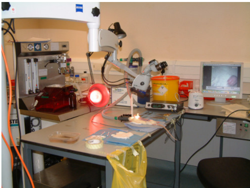
Figure 1. Equipment set-up. The anesthetic rig with red induction chamber are seen behind desk. The rat is lying supine with anesthesia maintained via a nose cone. A heat lamp is employed to increase ambient temperature. Above the rat is the operating microscope. To the left of the rat is a sterile drape with gauze, sutures etc. To the right of the rat is a sterile drape with the surgical instruments. Core temperature is maintained using a homeothermic blanket (underneath the rat) and rectal probe attached to the Harvard apparatus device (black box in front of the sharps bin).
