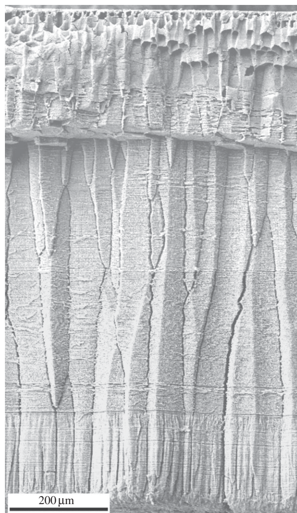
Figure 1. SEM view of a fracture of the calcitic prismatic layer of Pinctada margaritifera . The outer shell surface is at the top and prisms grow to the shell interior (downwards). During shell growth, many small prisms disappear, whereas the surviving units increase in size. Note organic walls surrounding prismatic units, particularly well preserved in the upper part of the layer.
