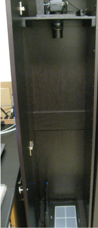
Figure 3. Imaging Cabinets. Imaging cabinets were specially built in our laboratory and used for high-throughput behavioral analyses. A 15 megapixel digital camera was attached to the top of the cabinet facing downwards in order to gather time lapse images of the larvae in multilane plates placed on top of the screen of a laptop. Between the plates and the screen there is a plastic diffuser that is used to prevent moiré patterns in the images collected.
