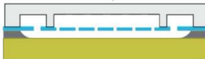
Figure 3. The microfabrication process of the biochip. The cell trapping and the sample delivery modules are microfabricated separately and subsequently exposed to air plasma, aligned and irreversibly bonded under an upright microscope.
