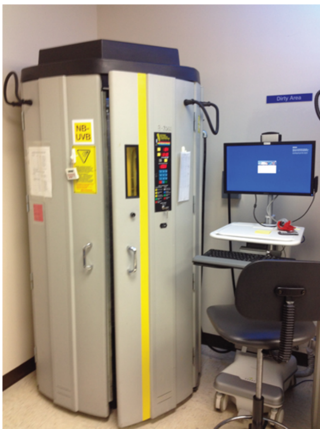
Figure 2. Narrowband UVB Station. Left is the narrowband UVB light box where patients enter and receive UVB phototherapy. Right is the attached computer station for the charting of phototherapy dosing and patient's response to phototherapy.
