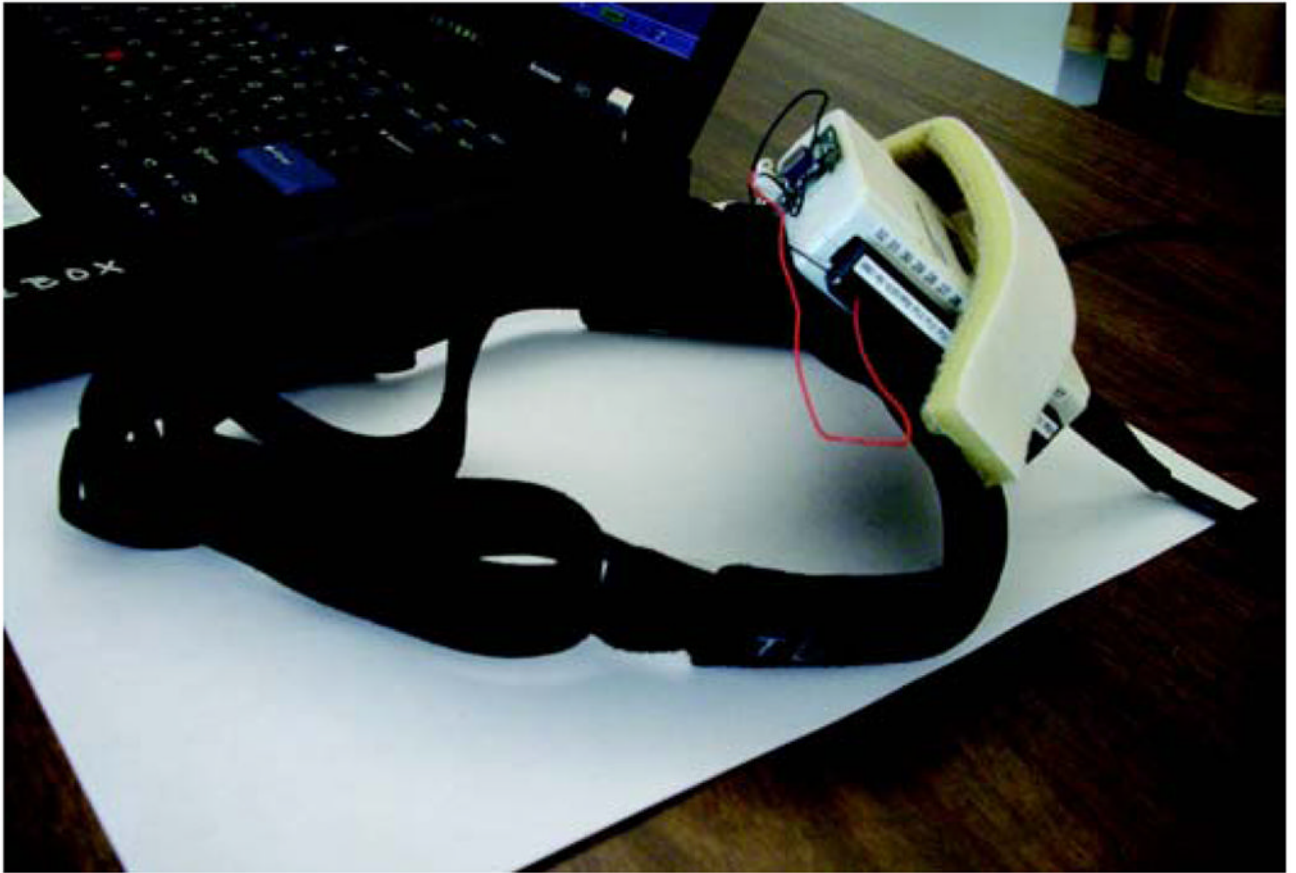
Figure 2. Dynamic visual acuity headgear. Rate sensor attached to headband.
