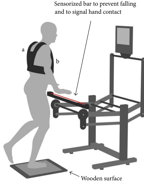
FIGURE 1: The postural proprioceptive station. The red line represents the infrared ray of the sensorized bar. Vest (a) to support the “postural reader”, (b) a two-dimensional accelerometer unit, in sternal position.
