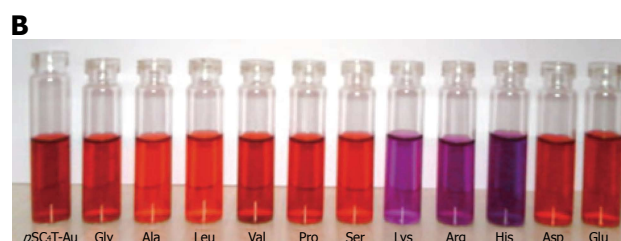
Figure 23 A is given a schematic representation of the amino acid induced aggregation of calix-capped gold nanoparticles; and in B are given the photographic images of calix-capped gold nanoparticles solutions containing different amino acids. From Patel et al [157] , reproduced with permission from Royal Society of Chemistry.
