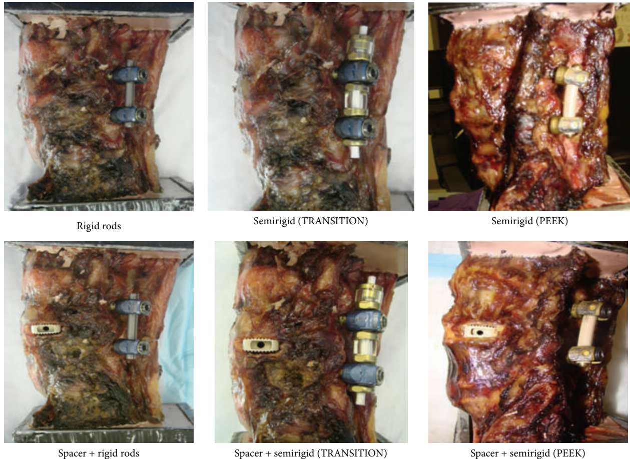
FIGURE 5: Select test images from flexibility testing, showing rigid and semirigid devices.
