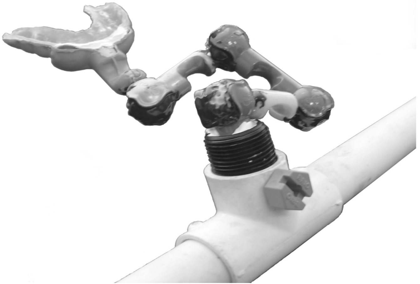
Figure. 1. Upper-jaw bite-bar mouthpieces were made for each subject and for each head position. They are attached to a bar that is firmly affixed to the sides of the dewar.
