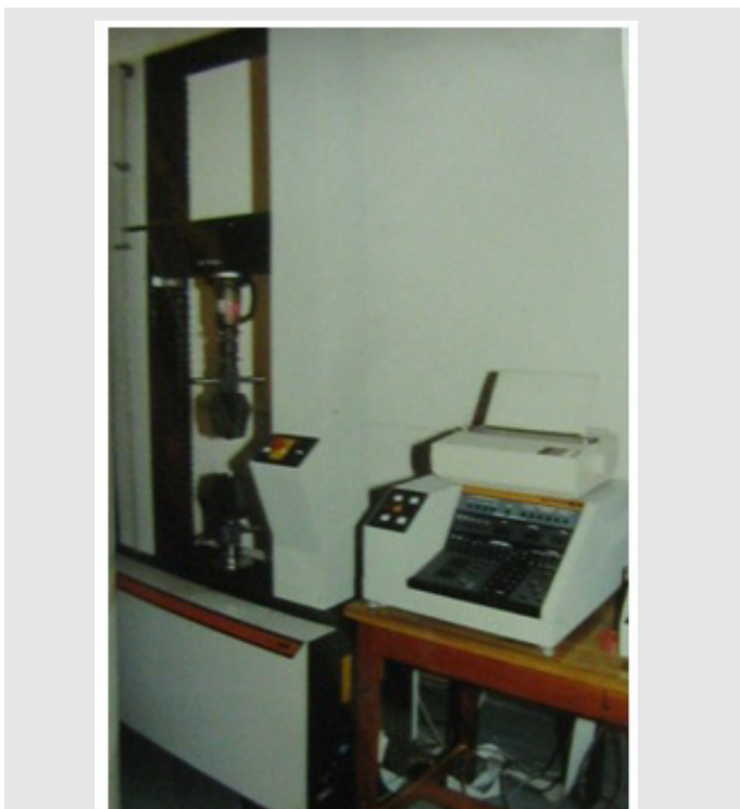
[Table/Fig-3]: Instron universal machine to measure shear bond strength
