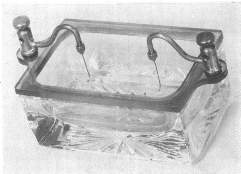
FIG. 6. THE CELL USED IN THE CAPILLARY TUBE METHOD
