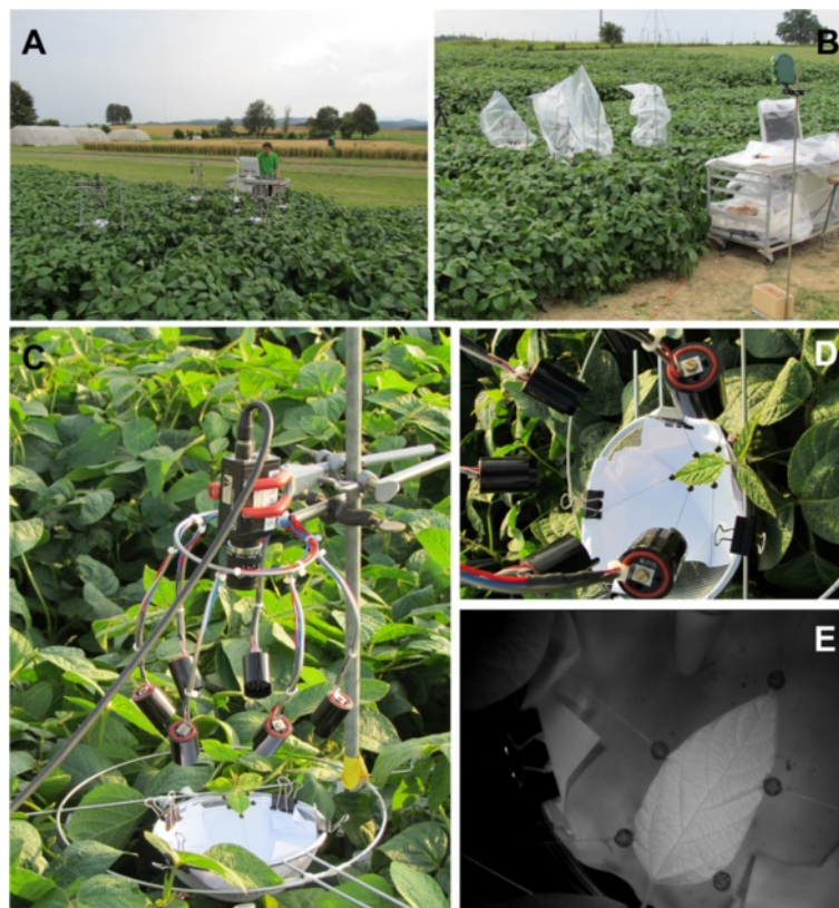
Figure 1 Setup used in the field. (A) Overview of the soybean field and setup; (B) Setup wrapped in plastic bags due to rain (measurement stopped); (C) Close-up view of the setup with infrared camera on top, infrared diodes and a soybean leaf fixed with strings glued to the leaf with attached weights; (D) Close-up view of the fixed soybean leaf with attached black beads; (E) Original image of a soybean leaf in the field taken with an infrared camera.
