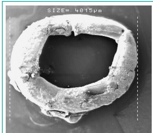
Figure 4 SEM micrograph of transparent elastomeric ligatures of ring type in latex (TR) after 4 weeks of permanence in oral cavity at original magnification x20.
