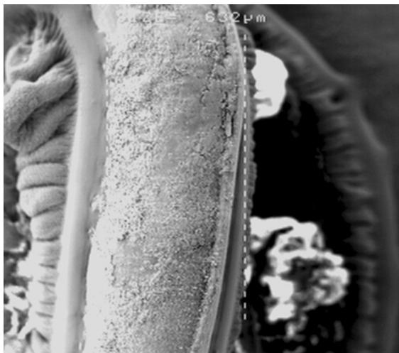
Figure 8 SEM micrograph of grey polyurethane Slide low-friction ligatures (GS) after 4 weeks of permanence in oral cavity at original magnification x50.
