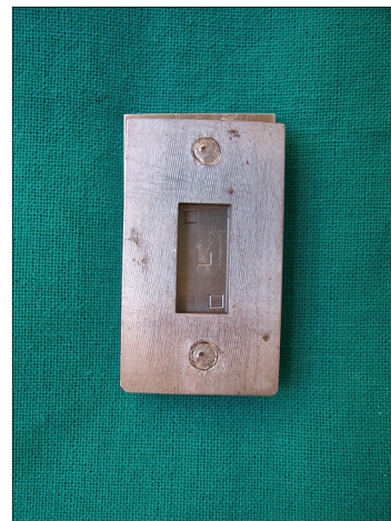
Figure 1: Photograph of brass metal mold
