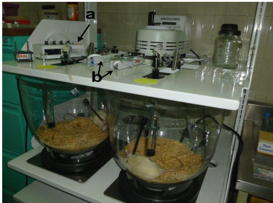
Figure 1. Representative images of microdialysis system for experimental models in vivo . The system consists of velocity controller (a) through which the vehicle is pushed; pumps (b) used for continuous infusion of analyte to be tested; the microdialysis cannula having an inlet tube (c); outlet tube (d) for recovery of the substance of interest; as well as clamping collar that is placed on experimental animals to have free movement (e); microdialysis cannule (f). Microdialysis system from Neurochemistry Laboratory of the Pediatric National Institute.
