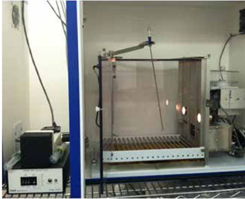
Figure 3. Standard operant chamber used for drug self-administration
