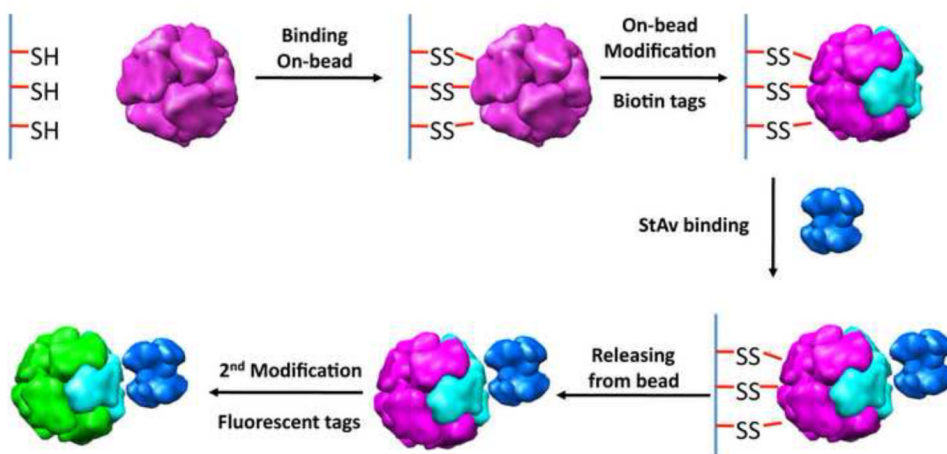
Fig. 12. Schematic illustration of a Janus-like LiDps cage preparation scheme through a masking/unmasking technique on a solid bead support [138]. The protein cages are first immobilized on beads through disulfide bonds. The exposed sides of the protein cages are modified with maleimide-PEG 2 -Biotin, which can selectively bind with streptavidin. Subsequently, the modified LiDps cages are eluted from the beads by reduction and the free cysteine residues on the cages are labeled with fluorescein-5-maleimide.
